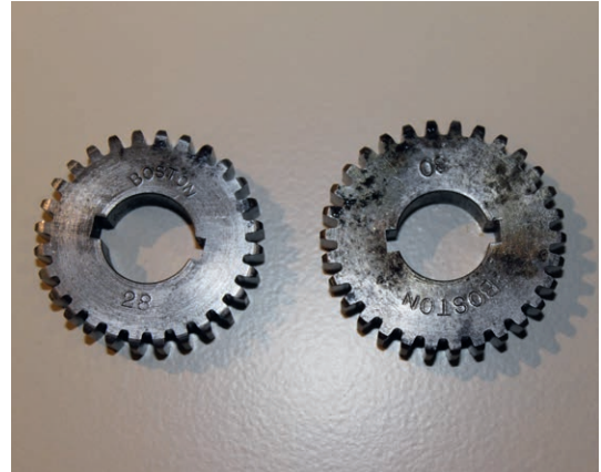
Fig. 10 – Two of the New York (Seewen) recorder's interchangeable cogwheels
