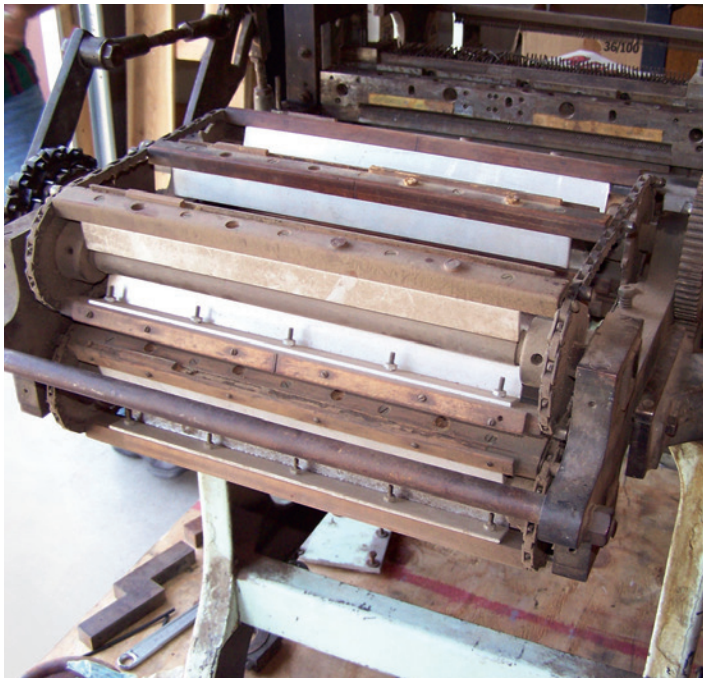
Fig. 11 – Paper tractor for making the commercial roll copies
