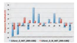
FIGURE 7 Comparison of frequency residuals (cent) versus note for "redesign" results of the Scherer\_O\_MET. The raw or unmodified results are in blue, while the modified wing joint results are in red.
