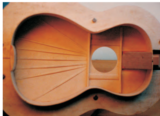
ILLUSTRATION 15 Fan bracing on a Panormo copy (copy by the author)
